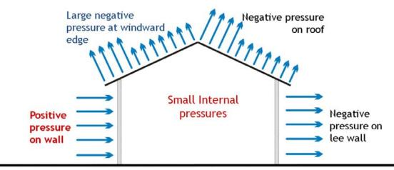
Figure 3 Representation of wind forces on a house
