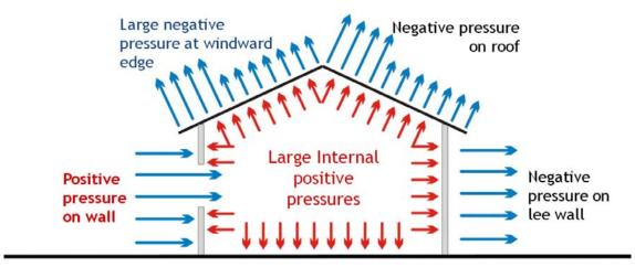
Figure 4 Wind forces with a dominant opening in windward wall
